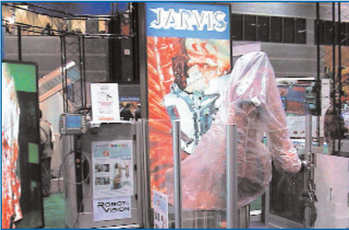
Display of one of the industrial robots Jarvis is now implementing for handling various kill floor operations. Protective covering over robot helps protect internal mechanisms from slaughterhouse corrosion.
